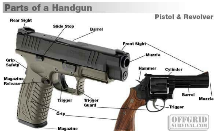
Figure 3.5: Parts of a hand gun
