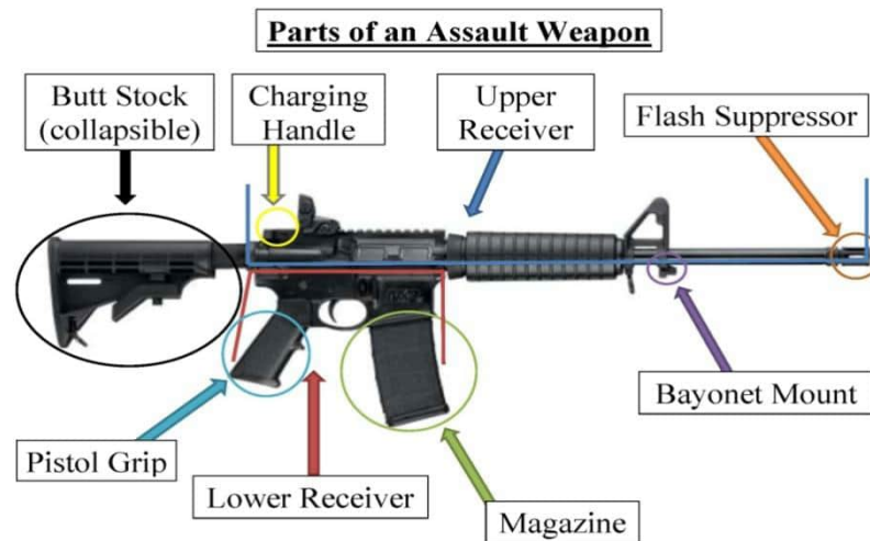
Figure 3.11: Parts of an assault weapon
