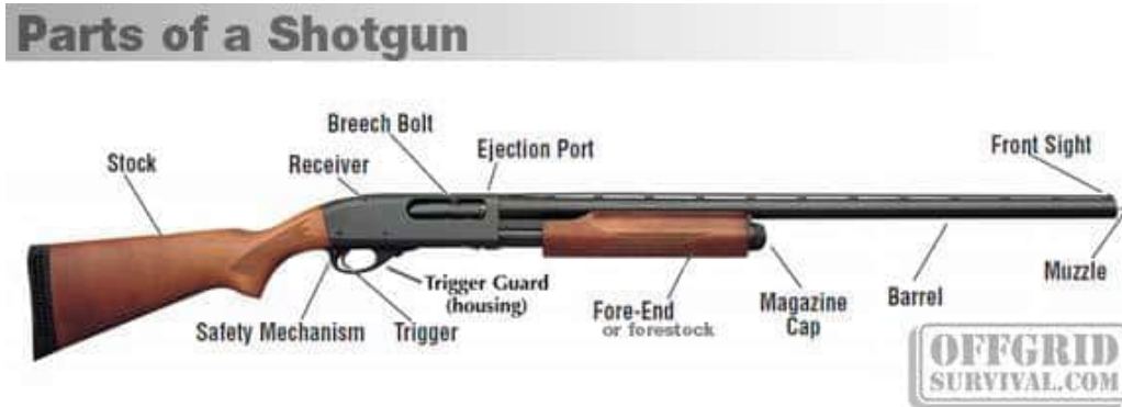
Figure 3.7: Parts of a shotgun
